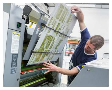
**Picture caption:** The new **Blackwood low chemistry UV plate** exhibits exacting dot reproduction, from 1-98%. With a simple 'wash out' bath, plates are press not only ready in seconds but the process minimises the consumption of chemicals and water.
