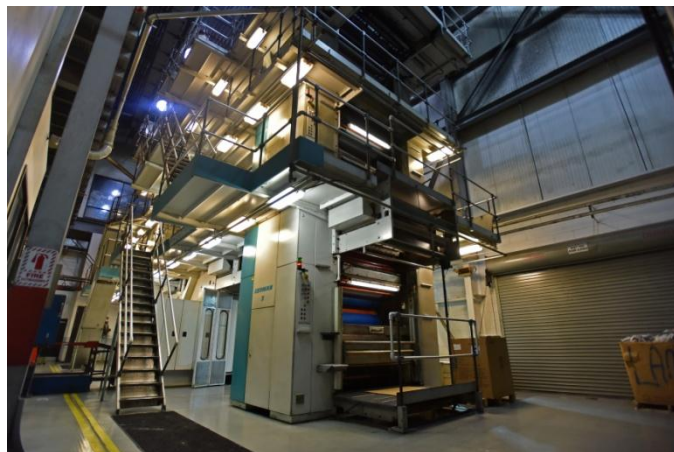
The manroland Geoman web press at the Wilkes-Barre newspaper printing facility was the first press of this type anywhere in the U.S.
