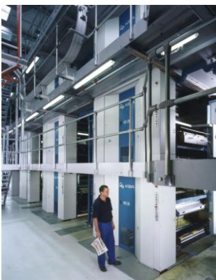
Production at Mediaprint takes place on a total of 13 KBA Commander web presses, which will be soon modernised as part of a major retrofit project
