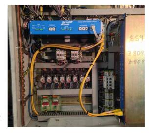
the on-unit ink, damp and registration (Z808 & 859) cards. In addition to the MPU upgrade, Harland Simon provided 22" press control touch screens for mounting on each Bargraph quality desk to enable quick adjustments of all press control functions.
