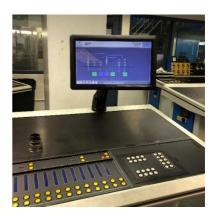
The new project at Butler Eagle involves replacement of the obsolete MPU with a PC based system which interfaces to the existing HDLC network, thus controlling the on-unit ink, damp and registration [Z808 & 859] cards. In addition to the MPU upgrade, Harland Simon will provide 22" press control touch screens for mounting on each Bargraph quality desk [see photo].
