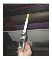
Semi-dynamic measuring is performed with the rollers moving at slow speed. This is the most real-life technique for analyzing a roller nip since the sensor blade detects both the flexibility of the roller rubber when it moves (viscous-dynamic properties) as well as the viscous-elastic properties (how the rubber hardens).
