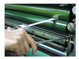
The top of the static sensor blade is inched into the nip and positioned between the rollers. A reading in millimeters or inches is shown. The pressman then easily can adjust the nip width to the level he desires. The static sensor blade detects the viscous-elastic properties of the rubber (how it hardens with age).
