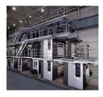
A 90,000-copies per hour *Goss Newsliner* press similar to two installed at Sankei Shimbun that are setting records for successful paper reel pastes.
