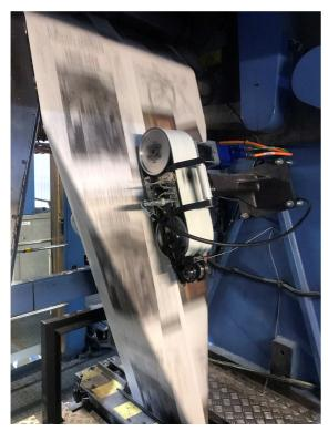
FLOWLINER Former When lateral stitching is performed on broadsheet products, the stitcher is mounted with one unit on each side of the former board.
