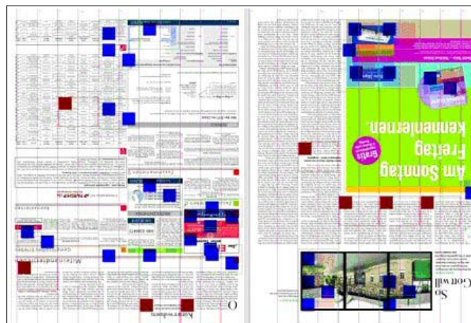
Example for the distribution of the so-called Regions of Interest (ROI) for the colour measurement which are automatically selected by the IDS.
