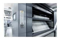
Specified with a *Goss Ecoset* dryer [pictured], *Contiweb FD* paster, *Goss Autoplate, DigiRail* digital inking and the *Goss Web Center* automated workflow and control system, the new press will also feature a PCF-3 combination and PFF-3 former folder, both designed to run at up to 100,000 copies per hour for optimum product versatility.
